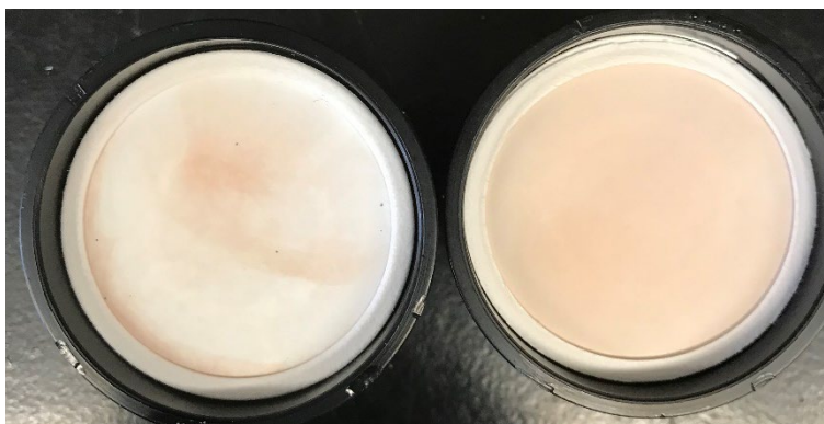
Figure 7. The comparison of brick slurry deposition pattern. Uneven distribution due to sequential addition (left) and even distribution using mixed addition (right).
