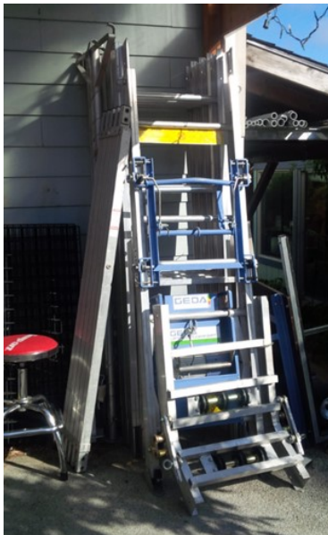
Fig. 12 Ladder hoists are recommended for panel lifting
