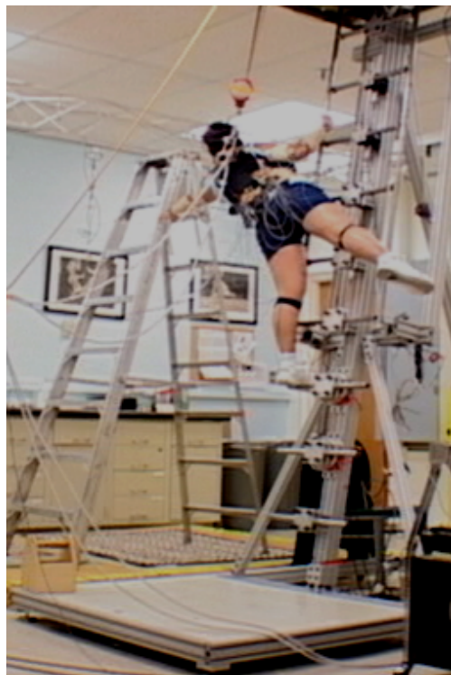
Figure 14: Photo of a subject reaching laterally to a target (the side of another ladder) one full arm span away from the center line of the ladder. The subject is holding the left rail.
