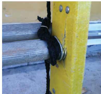
Figure 2: Damaged portable ladder
