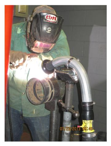
Figure 3: Welding carbon steel with LEV
