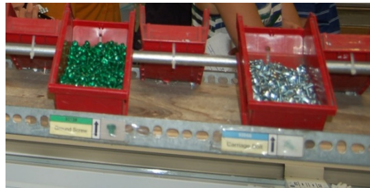
Figure 4: Color-coded Screws (and Corresponding Bin Labels) are Easy to Match/Tell Apart (facilitate recognition) (Source: Iris Tommelein)
