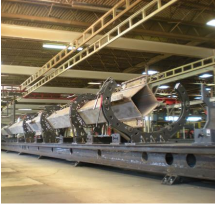
ConXTech fabrication shop with rotating clamps www.prweb.com/releases/conxtech/ladbs-approved/prweb10762433.htm
