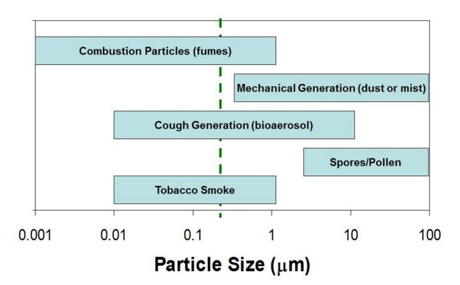
Note: The dashed green line represents the 0.3 µm mass median aerodynamic diameter (MMAD) sodium chloride aerosol used by NIOSH for respirator filter testing of N95-class air-purifying respirators.
