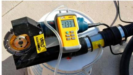
The vacuum weighs 103 pounds and is specified to provide 258 cubic feet of air flow per minute (cfm) and a "static lift" or "vacuum suction pressure" of 100 inches of water. The vacuum includes a cyclonic preseparator, which removes larger particles, a pre-filter (rated >99.5 percent efficient) and two high-efficiency particulate air (HEPA) filters (which by
