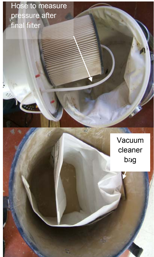
Figure D-1. Locations for measuring static pressures inside the Dust Director vacuum cleaner. After sucking 5 pounds of debris into the vacuum cleaner, the vacuum cleaner hose was removed and manometer hose was inserted into the bag. Also, holes were drilled in the body of the vacuum cleaner tank and hoses were inserted into the spaces between the filters. And after the final filter.
