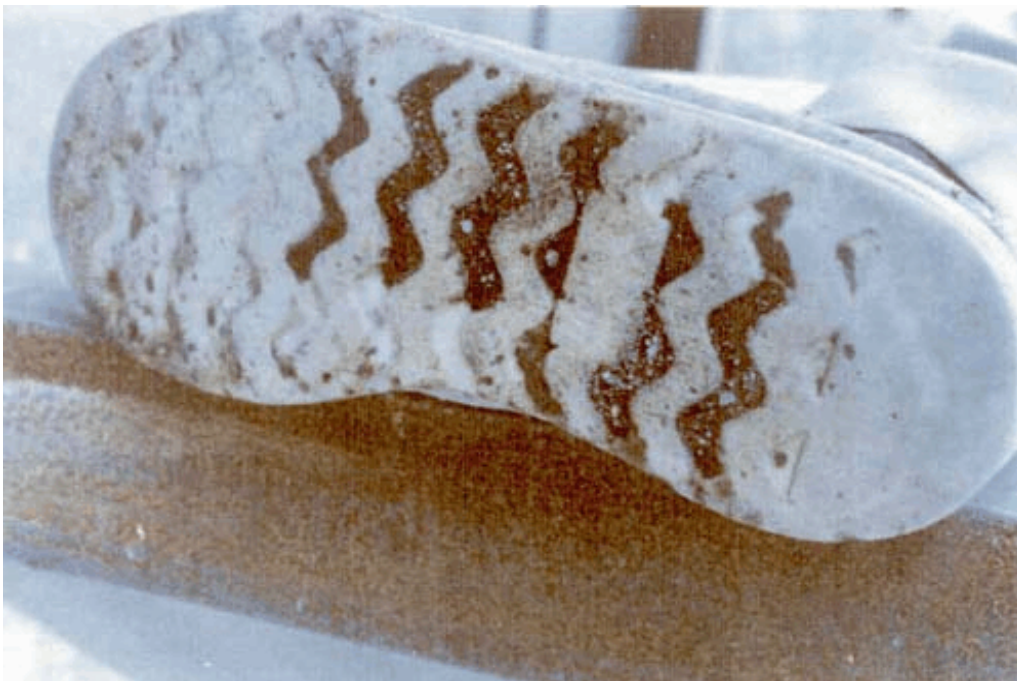
Figure 12. Contamination was removed from the bottoms by sanding.
