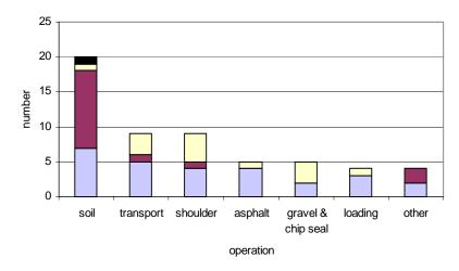
**Figure 5.** Number of compactor overturns resulting in operator injury, by conditions and type of compactor, 1985-2002 *Note:* 56 cases
