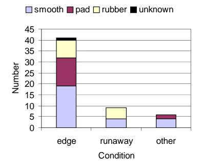
**Figure 7.** Conditions contributing to overturns, by type of compactor and number of overturn incidents, 1985-2002 *Source:* Based on OSHA and NIOSH reports
