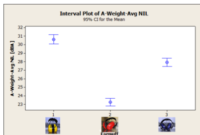
Figure 7: 95% Confidence Intervals for A-Weighted Average NIL versus Earmuffs From Figure 6, we can also observe that protective eyewear 4 and 5 were associated with the highest and lowest earmuff noise insertion loss respectively as depicted in Figure 8 with the 95% confidence intervals for the NIL in dBA versus eyewear.
