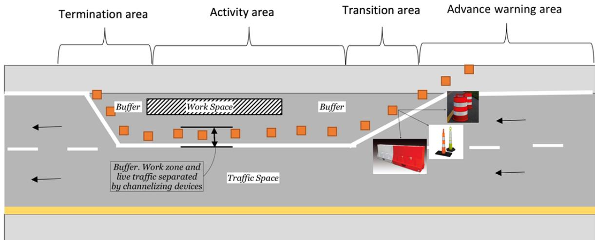
**Figure 1. Basic highway construction work zone layout (Adapted from ITSI, 2011)**
