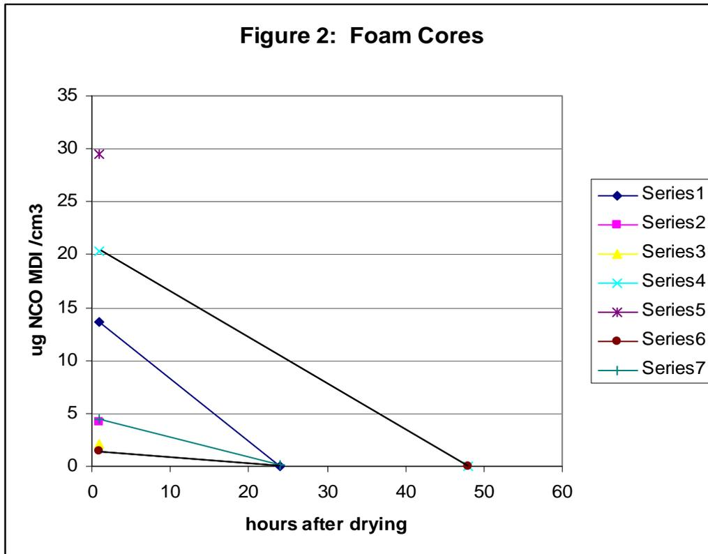
In addition to qualitative and quantitative surface wipe samples, we also used punch biopsy tools to extract cores from the foam product. These cores of the full thickness of foam were taken 60 minutes, 24 and 48 hours after application. To date 11 core samples have been analyzed by Dr. Bello to determine the amount of free isocyanate in the product.
