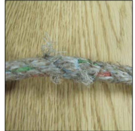
Photo 4. Damaged fibers in laborer's 50-foot lifeline (Photo courtesy of NCDOL/OSH)
