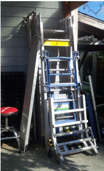
Fig. 12 Ladder hoists are recommended for panel lifting
