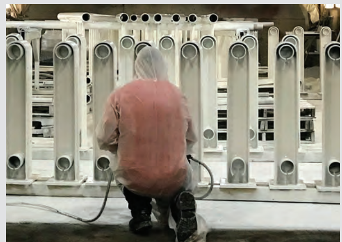
A painter applying a polyurethane topcoat on decorative railings and small bridge parts.
