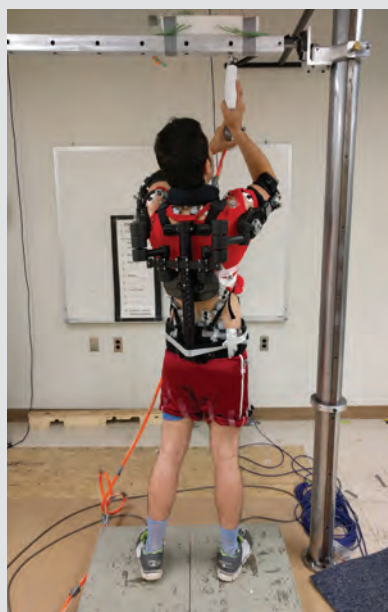
Examining the impact of passive exoskeletons in improving construction worker safety and health in the lab at Virginia Tech.
