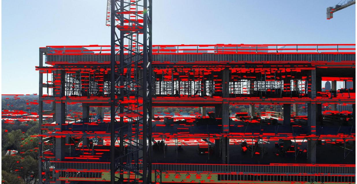
**Figure 7: Visualization of the detected horizontal line segments**
