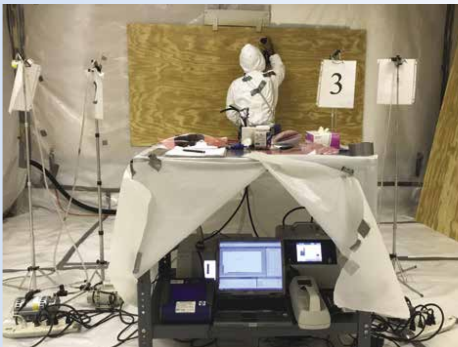
View of real-time instruments for measuring particles generated during spraying and sanding of paints and coatings.
