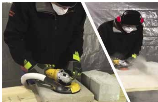
Angle grinding, with and without dust capture.
