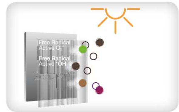
3 Free radicals are formed by the transferred energy ( \text{O}_2^- , \bullet\text{OH} ).
