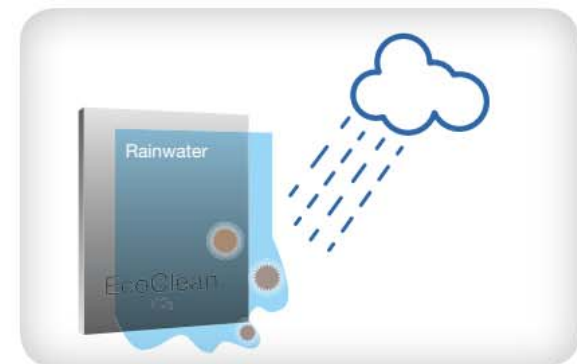
6 The hydroxyls make the building surface super slick. Instead of beading up on the surface, the water collapses on the surface and runs off, undercutting dirt and grime.
