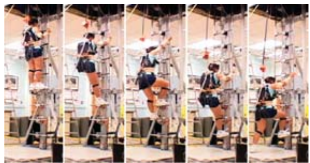
A specially built ladder and infra-red motion tracking system were used to record movements up and down a fixed ladder in a lab setting.
