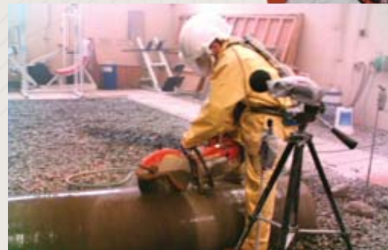
A laborer cuts a concrete pipe at the New England Laborers Training Center to test noise levels of a blade and gas-powered saw.
