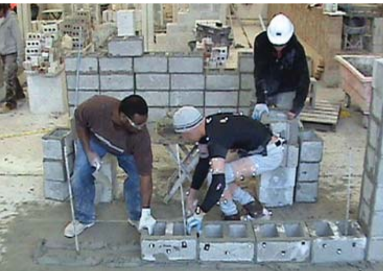
Masons participated in Dr. Anton's tests to examine muscle use when lifting concrete block. The white dots indicate the sensors reading the mason's muscle activity.
