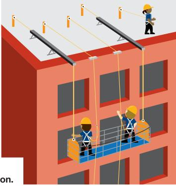
**Engineered anchor point systems typically** exceed regulations and are the safest option.
