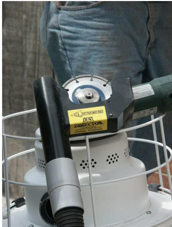
Figure 1. Metabo grinder with Dust Director shroud
