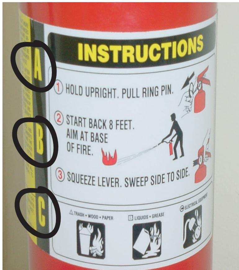
The same label also includes information on the amount of dry chemical stored in the extinguisher. The number in front of the A indicates how much water the extinguisher is equal to and represents 1.25 gallons of water for every unit of one. In this case, a 3-A rated extinguisher would be equal to 3.75 gallons of water (3 x 1.25).
