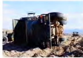
A dump truck rollover that occurred while operating on a soft surface.
