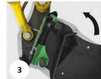
3 Accidentally opening a quick coupler in an unsafe position
