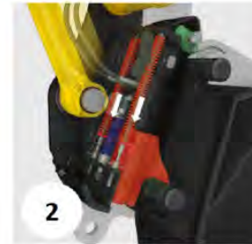
2 Cylinder failure / Loss of hydraulic pressure
