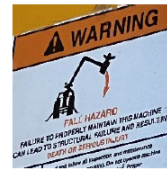
Fall hazard warning label on base of boom lift.
