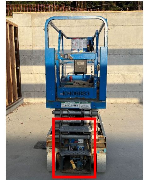
Photo 2. Rear view of lift with steps shown in red outline.
