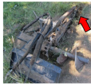
Trencher attachment. Arrow shows chain and digging teeth.
