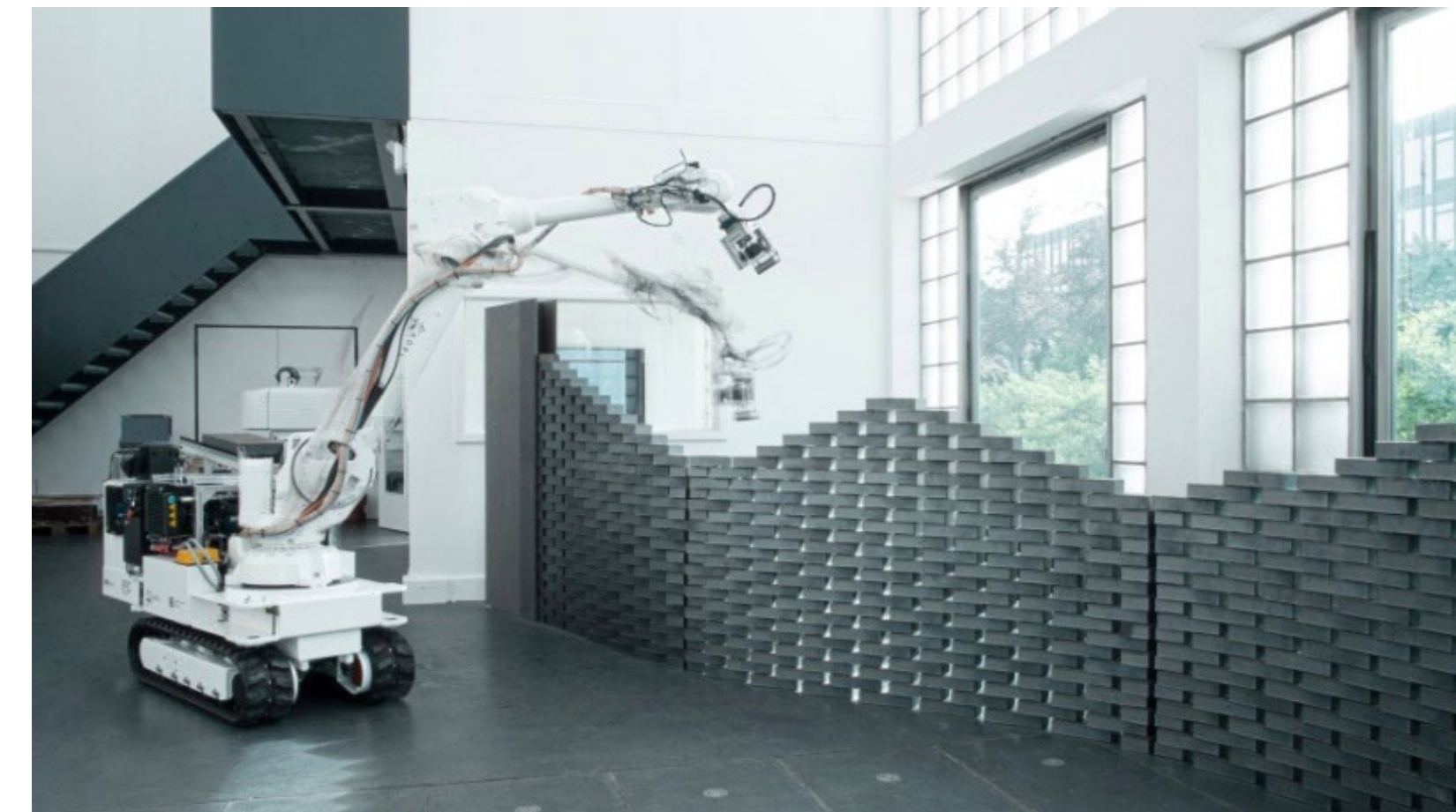
Mobile robotic fabrication (Gifftthaler et al. 2017)
