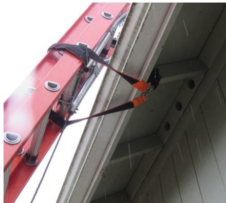
Fig. 13 Ladder stabilization device
