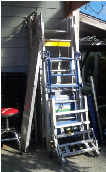
Fig. 12 Ladder hoists are recommended for panel lifting
