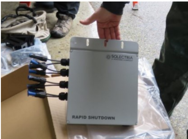
Fig. 16 Rapid shutdown device for a residential project
