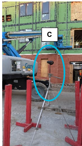
Figure 1: Noise exposure measurement setup, with dosimeter (A: red), SQobold binaural headset and DAQ system (B: yellow), and sound level meter (C: blue)
