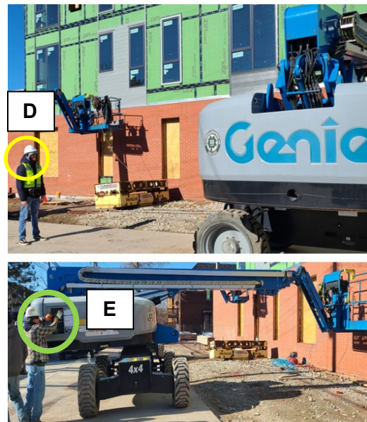
Figure 2: Audibility of warning signals, measurement setup with siren sound emission adjustment (E: bottom/green), and SQobold binaural measurement around the equipment (D: top/yellow)
