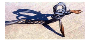
(10)(iii): broken wires
