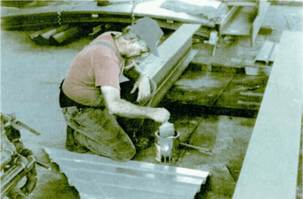
Figure 2. Experimental paints were all applied by brushing by an ADF employee.
