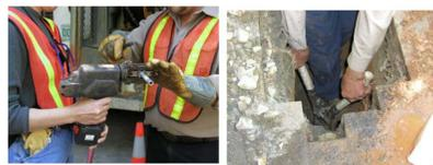
Direct buried cable battery (left) and manual tool (right)
