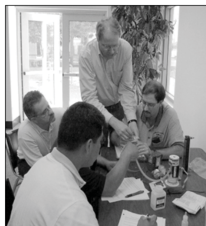
Union health & safety trainers learn from a certified industrial hygienist how to calibrate a personal sampling pump. Arrow points to calibrating device.
