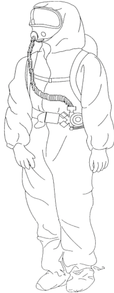
A Level B suit that covers the SCBA would reduce equipment contamination
