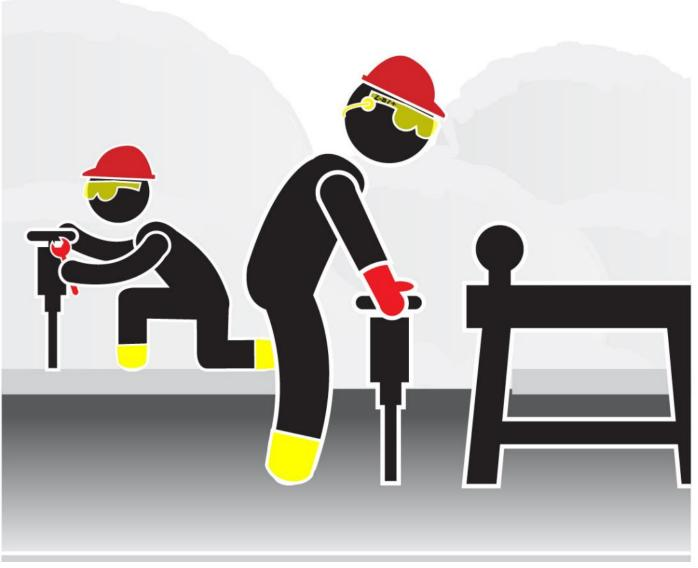
Wear gloves or use anti-vibration wraps to improve grip strength and lessen the shock of vibrating tools.
