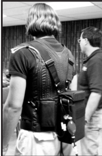
A closer view of the vest, bottle carrier (r), pump priming bulb (m), and battery pack (l)
