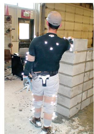
*Motion capture sensor markers attached to a bricklayer's clothing record back and arm positions to detect stressful work positions.*
