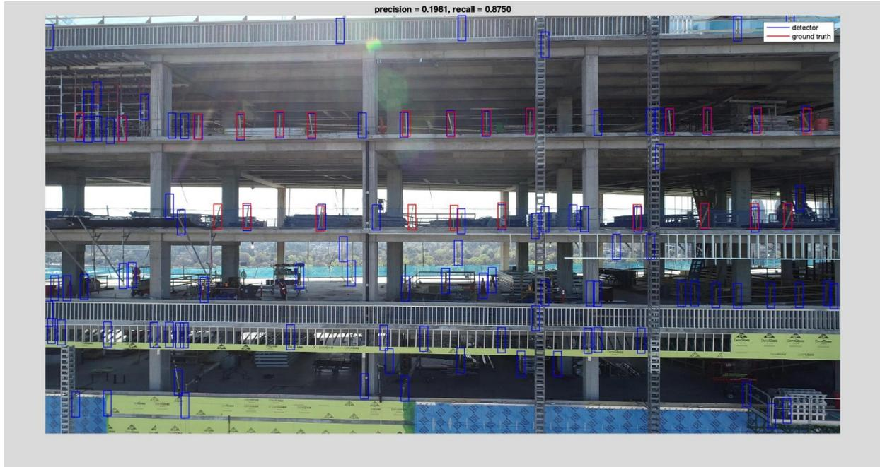
**Figure 11: Visualizations of the guardrail detections using linear SVM**
