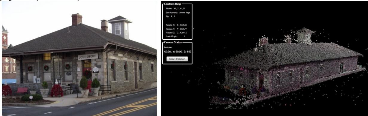
**Figure 1: Sample of a generated PCD for a building (Rashidi et al. 2013)**
