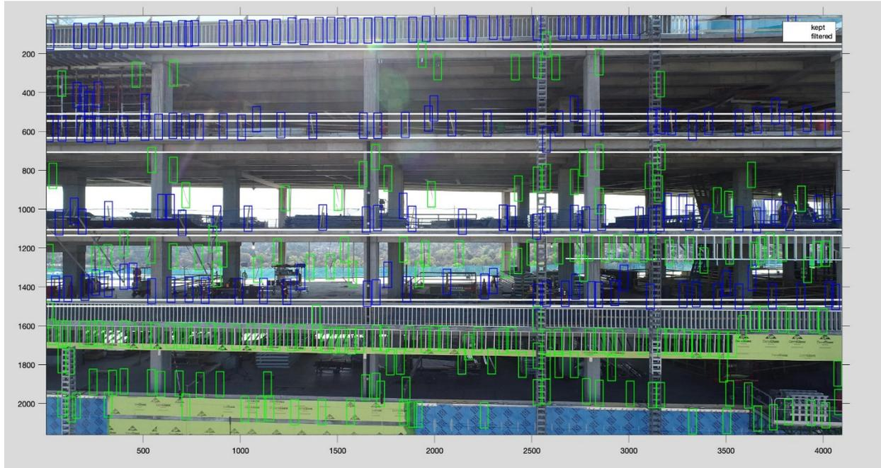
**Figure 13: Visualization of the filtered false positive windows (denoted as green bounding boxes). White lines are the detected floors.**
