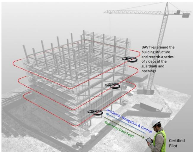
Figure 5: A conceptual illustration of capturing videos of a high-rise construction projects using a quadcopter
