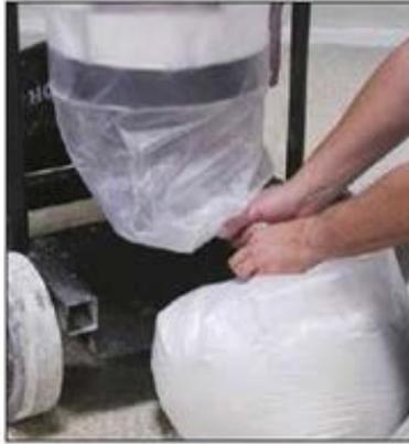
Continuous plastic tube is pulled downward and divided in single bags of any size.
