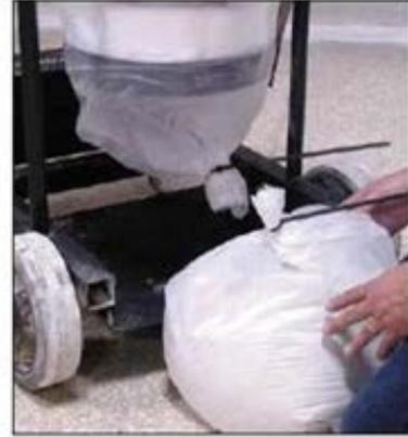
Cut between the ties and dispose the filled bag.
