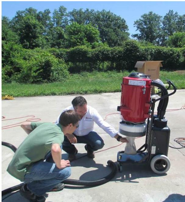
leaving one tie in place at what will be the bottom of the next dust collection section. Use of the continuous tube allows the tuckpointer to tie off a section loaded with dust and cut it off without having to remove or replace any bags attached to the vacuum and can be removed relatively quickly and easily without exposing the operator to its contents.
