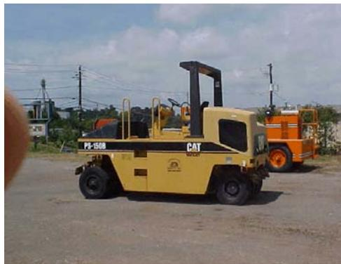
**Figure 3.** A rubber-tired compactor with a two-post ROPS.
