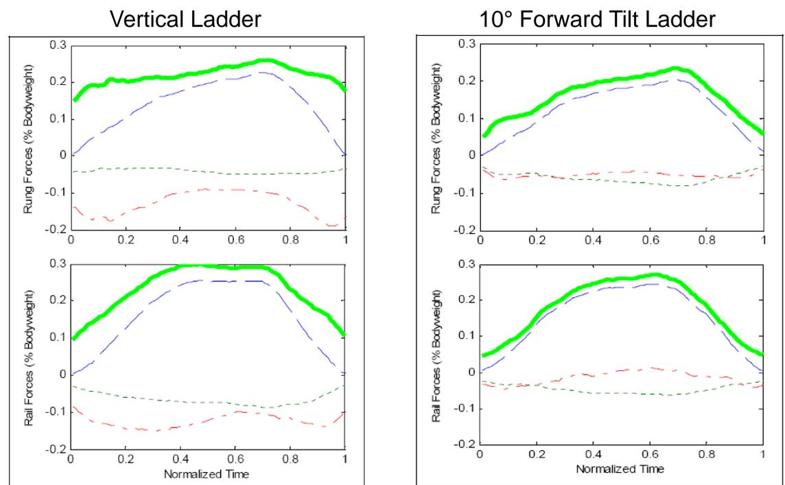
Component forces are dominated by lateral forces (x), but on the vertical rail, in/out (z) forces were larger during the initial reach and the return phase of the exercise. This was not the case for the tilted ladder.
