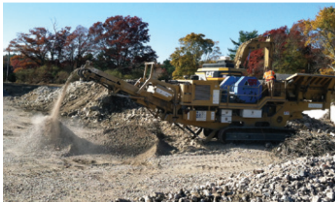
Rock crushing (above) creates high levels of silica exposure, but researchers found misting equipment provided valuable protection to workers.
