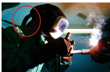
A respirator protects this welder—the respirator hose is circled in red.
