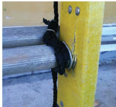
Figure 2: Damaged portable ladder
