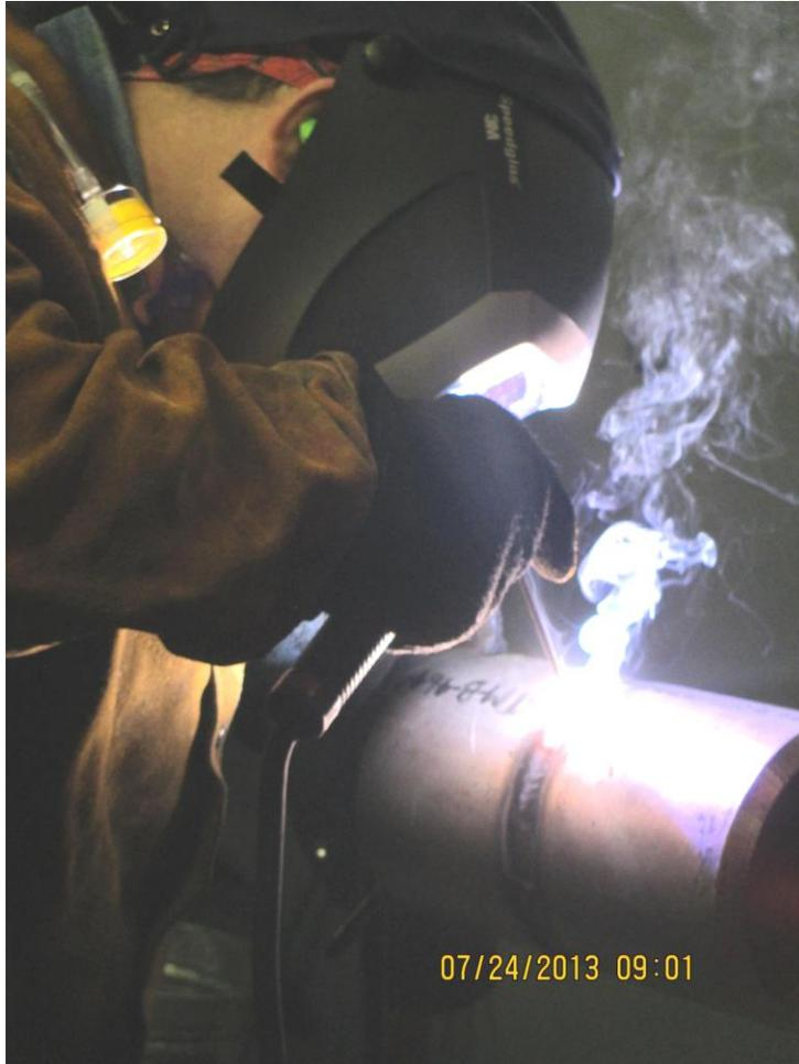
**Carbon/mild steel welding.** Carbon steel schedule 80 each pipe welds consisted of two passes: a root pass followed by a fill pass. Shielded metal arc welding was used for both the root pass (6010 electrode; 1/8”), and the fill pass (7018 electrode; 3/32”). It was noted that trials that included the root pass were not equally distributed between no-control and LEV control trials.
