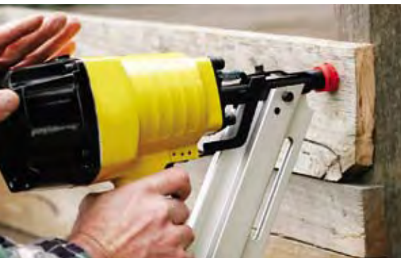
Nail gun injury rates decreased when use of sequential triggers and training increased.
