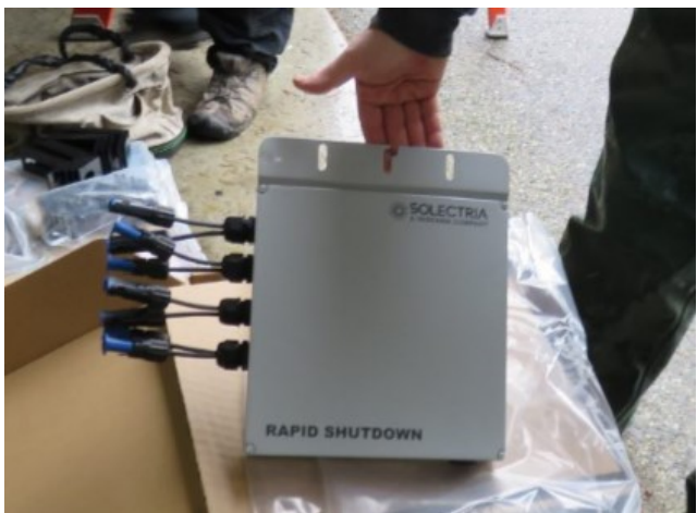
Fig. 16 Rapid shutdown device for a residential project
